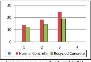
Fig 6. Compressive strength of Normal & RCA concrete.
