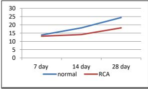
Fig 7. Reduction in Compressive Strength.
