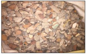
Fig 3. Recycled Coarse Aggregate.
