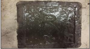
Fig 4. Recycled Aggregate Concrete Casted Cube.
